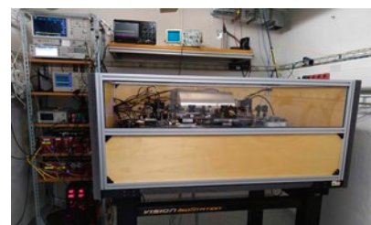
High-finesse optical cavity for sub-Hz linewidth laser
