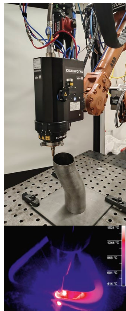
Fig. 3 WLAM: Robotic arm with CoaxM 3D printing head for the WLAM technology and an example of 3D printed specimens. Embedded image: SWIR camera capture of print detail.
