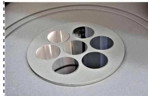
Example of an Ag-based laser mirror on a glass substrate.
