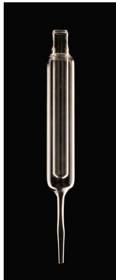
Scientific glassware workshop: Dewar bottle for cryogenics
