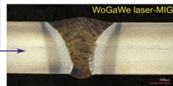
Fig. 2 Hybrid: Conventional hybrid laser-MIG welding often produces an inhomogeneous weld metal (upper macrograph). This issue is addressed by the new WoGaWe technology (schematic and lower macrograph), which produces a more uniform weld structure (S700MC, sheet thickness 5 mm, welding speed 15 mm·s -1 ).
