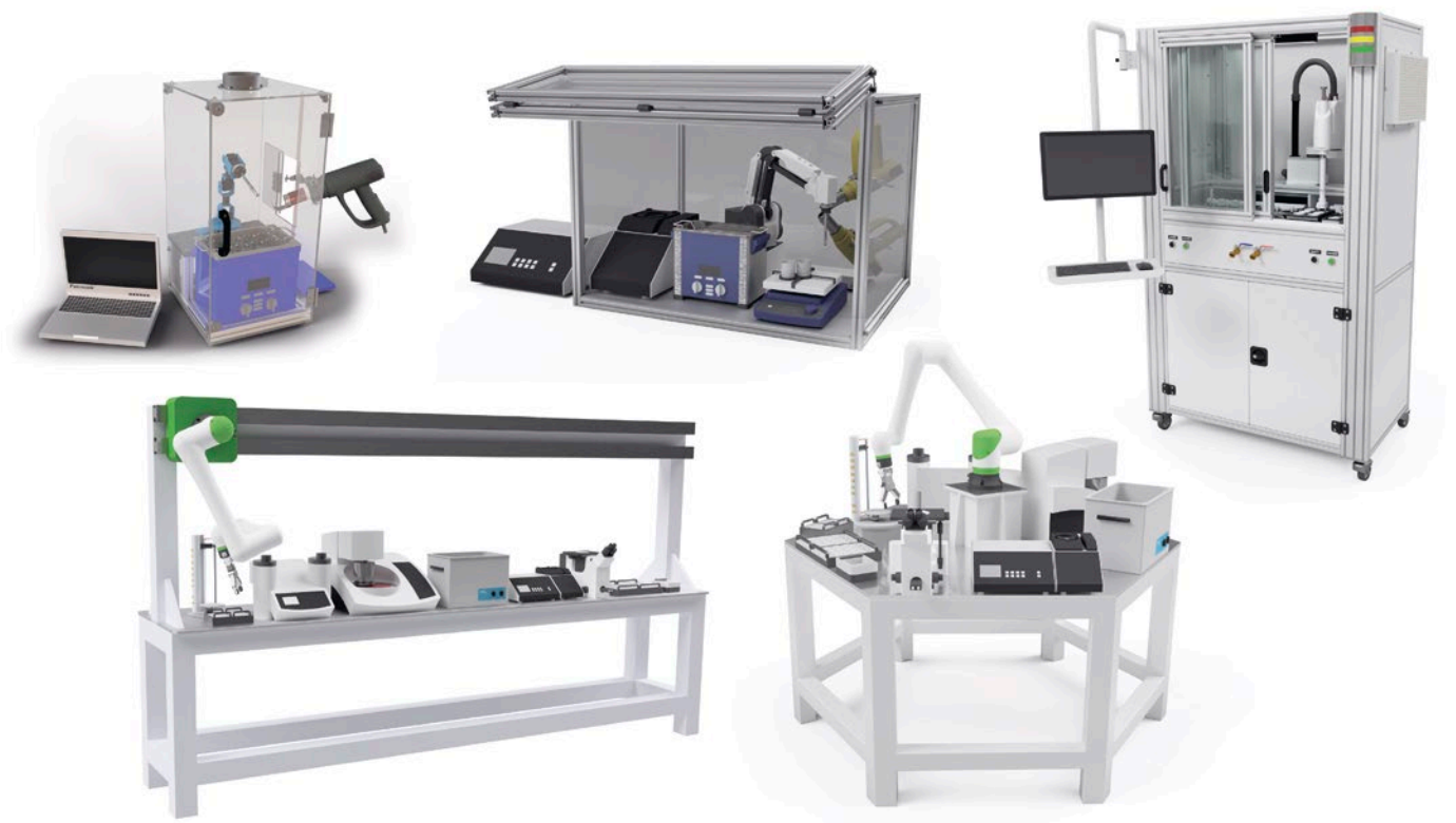
Robotic concepts for reducing the stochasticity, workload and danger in metallographic sample preparation
