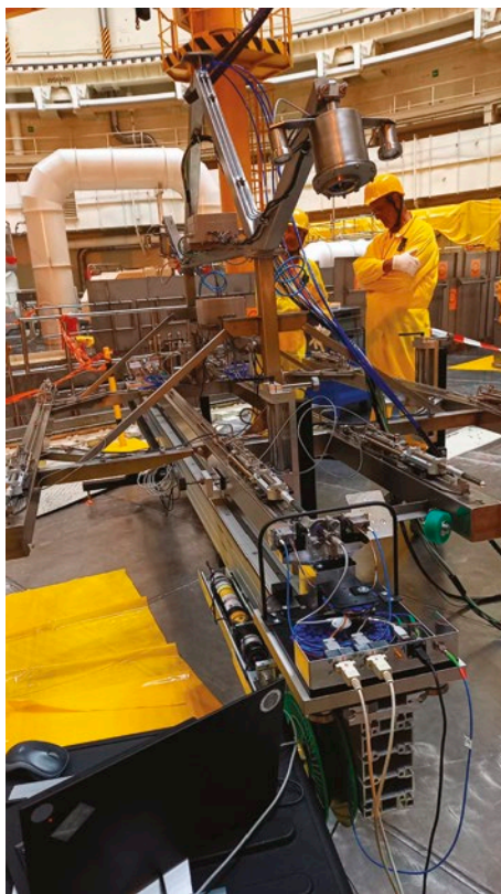
Specialized interferometric test-bench for calibration in the nuclear power plant reactor hall.
