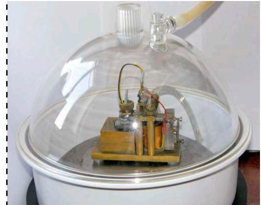
Impact tester in chamber with controlled atmosphere
