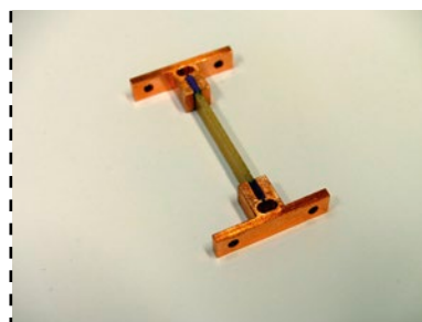
Example of an epoxy composite sample for thermal conductivity measurement in our dedicated apparatus.
