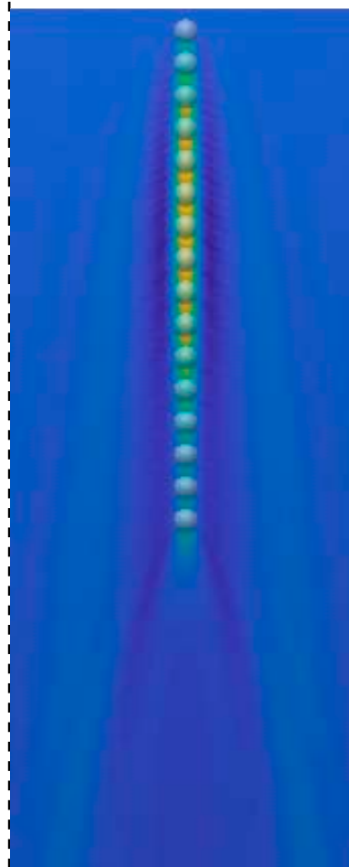
Example of optical sorting of suspension of polystyrene particles of sizes 800 nm and 1600 nm in travelling interference fringes
