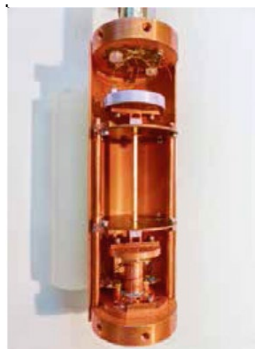
Apparatus for measurement of thermal conductivity of metallic and non-metallic materials
