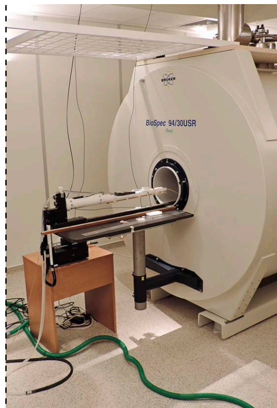
Biomedical 9.4T MR scanner equipped for mouse, rat and rabbit imaging
