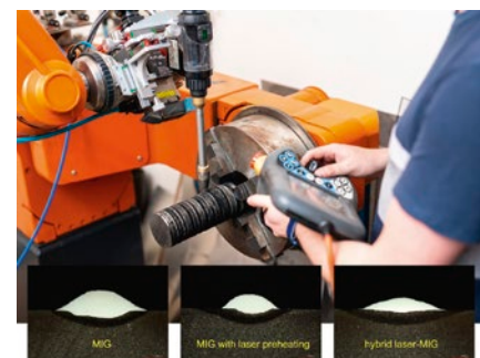
Fig. 4 Cladding: Cladding of cobalt-based alloy on creep-resistant steel and a comparison of bead geometry for different cladding technologies at constant total power 4.2 kW and welding speed 40 mm·s -1 .
