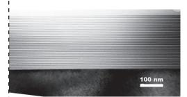
Cross section of the Si/C multilayer on silicon substrate
