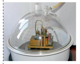
Impact tester in chamber with controlled atmosphere
