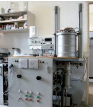
Laboratory vacuum furnace built at ISL
