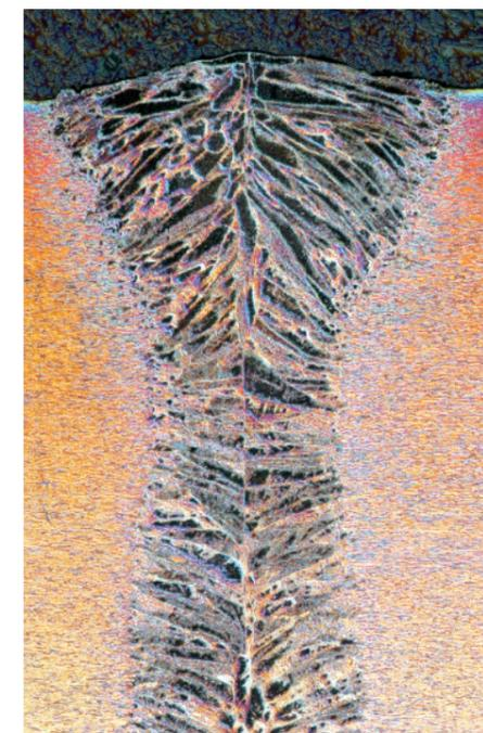
*The section of the laser weld visualised by Nomarski method.*
