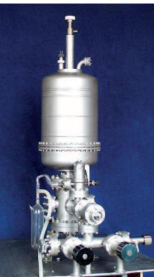
Helium bath cryopump for ultra-clean pumping of vacuum spaces without vibration and electrical power.
