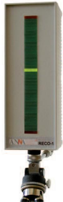
**RECO – device for respiration control.** LEDs bargraph for pacing of breathing. It is used for controlled excitation of the cardiovascular system. It enables setting of pacing frequency 1–39 min<sup>-1</sup>, various modulations – ramp and sinus with depth of 25–100%.
