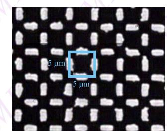
CCD camera was first calibrated using lithographic mask with spacing between grooves equal to 5µm. We obtained that one pixel corresponded to 62.5 nm using objective Olympus UPlanFl 100x/1.3 Oil Iri and 1/3` CCD chip (CCD camera Kampro KC-381CG).
