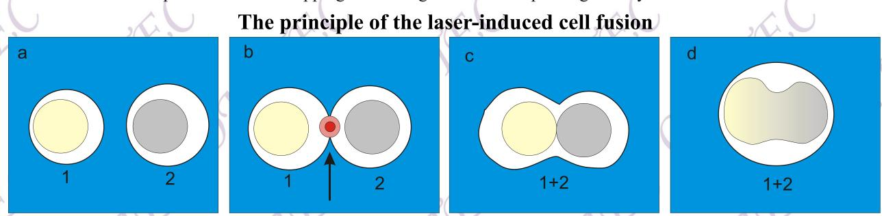
(a) Two cells (denoted as 1, 2) are brought into contact using optical tweezers. (b) Laser pulses are applied to perforate the cell membrane at the point of contact (denoted by arrow). (c) The content of both cells is mixed. (d) The nuclei fuse together and the fusion product takes round shape again.
