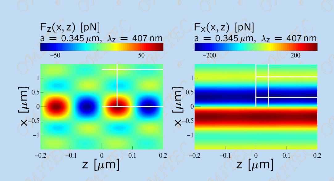
Optical forces acting on micro-particles placed in standing Bessel beam were counted by use of the Barton's method. It has been shown that the equilibrium position of these spheres centre is in the intensity maximum along x axis but in intensity minimum (standing wave node) along z axis.
