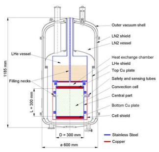
Cryostat conception is based on our long-term experience in cryostat design, especially low-loss cryostats for NMR magnets.
