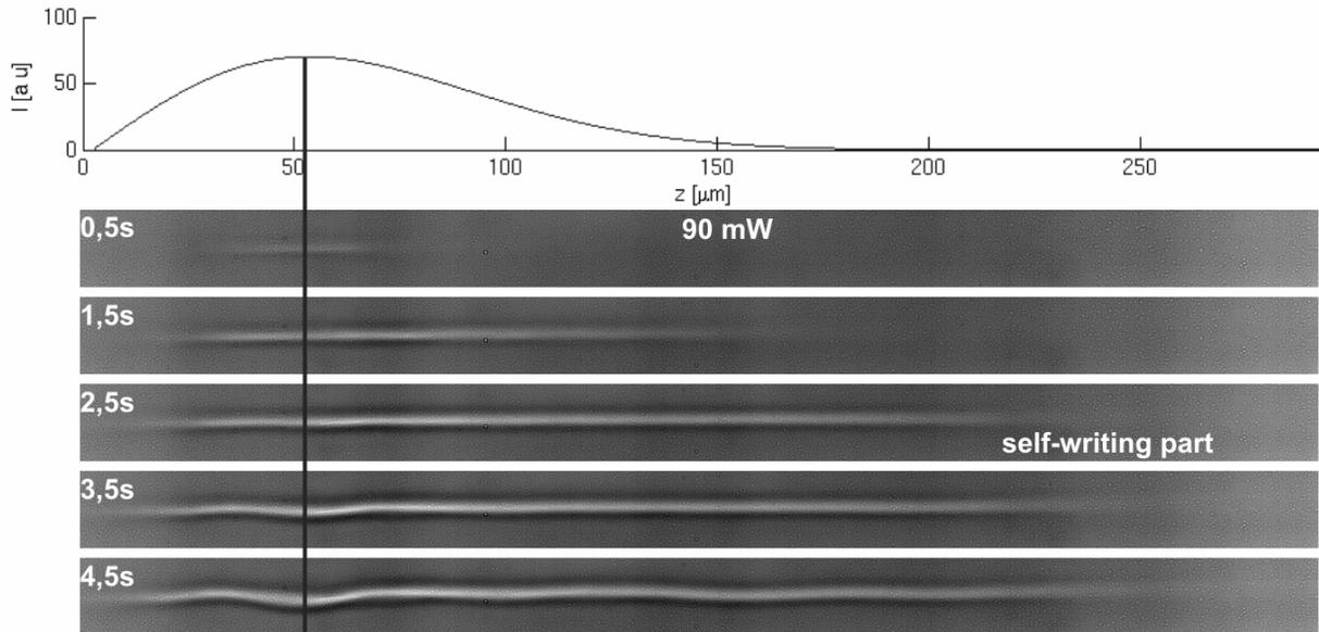
**Fig. 4.** Formation of the polymer fiber in the short BB. The BB core radius was  $0.8$   $\mu\text{m}$  and the maximum propagation distance of the BB was about  $100$   $\mu\text{m}$ . The laser power in the cuvette was  $90$  mW. The top plot shows the calculated on-axis intensity profile of the BB for the parameters used in the experiment.
