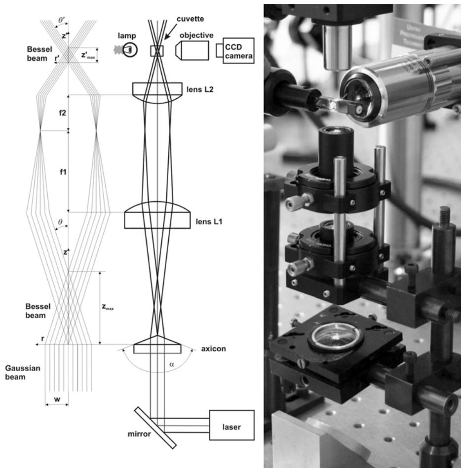
**Fig. 1.** Optical setup for creation polymer fiber by photopolymerization and by Bessel beam.
