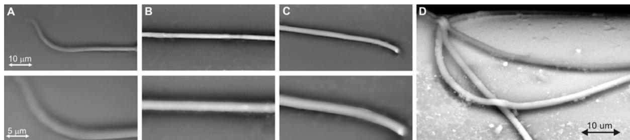
**Fig. 3.** ESEM images of the left (A), middle (B) and right (C) part of one fiber long 15 mm (see the column B in Fig. 2.). Each of the image rows keeps the same scale but uses different magnifications to demonstrate the fiber homogeneity. The
