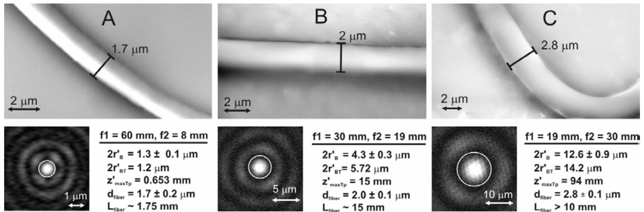
**Fig. 2.** Top row: ESEM image of the polymer fibers. In all three cases we used the same output laser power 3 W giving laser power 1.5 W in the cuvette. Bottom row: Lateral intensity profiles of three types of generated BBs with different diameters of the BB cores ( $2r'_B$ ). Corresponding parameters of the set-up, created fiber diameter ( $d_{\text{fiber}}$ ), and its length ( $L_{\text{fiber}}$ ).
