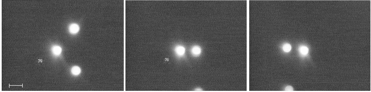
Figure 7. Manipulation with fluorescently labelled polystyrene particles (denoted by arrow) trapped by LMA1, trapping power 30 mW. Vector on the first picture has length 5 \mu\text{m} .
