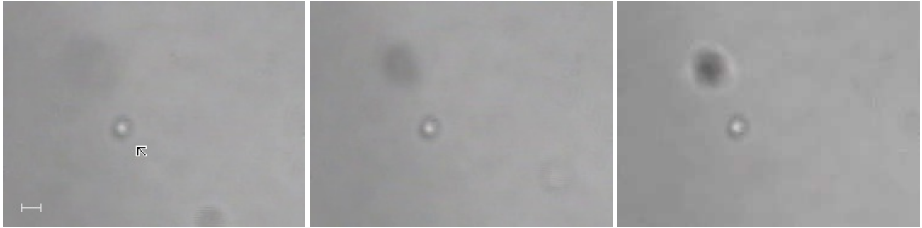
Figure 4. Arrow signed polymer microsphere with diameter 520 nm (3k-500 Duke Scientific) in water solution is trapped by LMA1. The position of the optical trap is changed by vertical movement of the microscope objective and image on CCD camera focuses. Power in the focal point is 55 mW. Vector on the first picture has length 1 \mu\text{m} .
