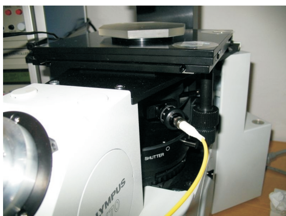
Laser microscope adapter (LMA 3) is placed into objective turret, into a space for e.g. Nomarski DIC slider
