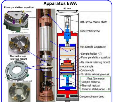
Whole apparatus is inserted in wide neck LHe dewar vessel.
